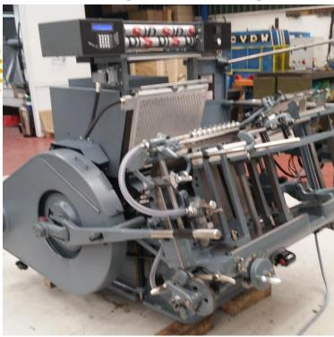
Heidelberg "GTP" 13"x18" (34cmx46cm) Platen foil blocking machine that has had the base unit completely refurbished. New foil pull conversion fitted
