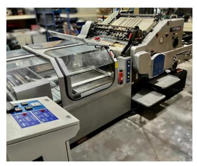
Heidelberg "SBD" 640mm x 900mm cylinder foil blocking machine that has had the base unit dismantled completely refurbished 2024 and replacing any part that is found to be damaged, foil pull conversion completely new, Toggle heated bed plate replaced.
